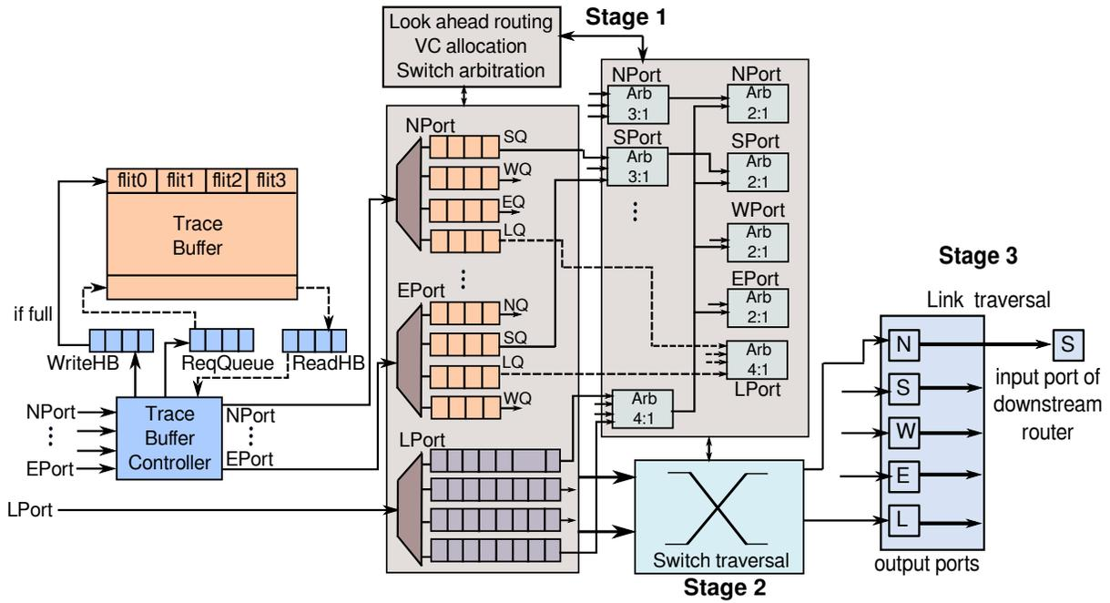
Fig. 5: Output Port Directed VC Assignment (ODVC)
