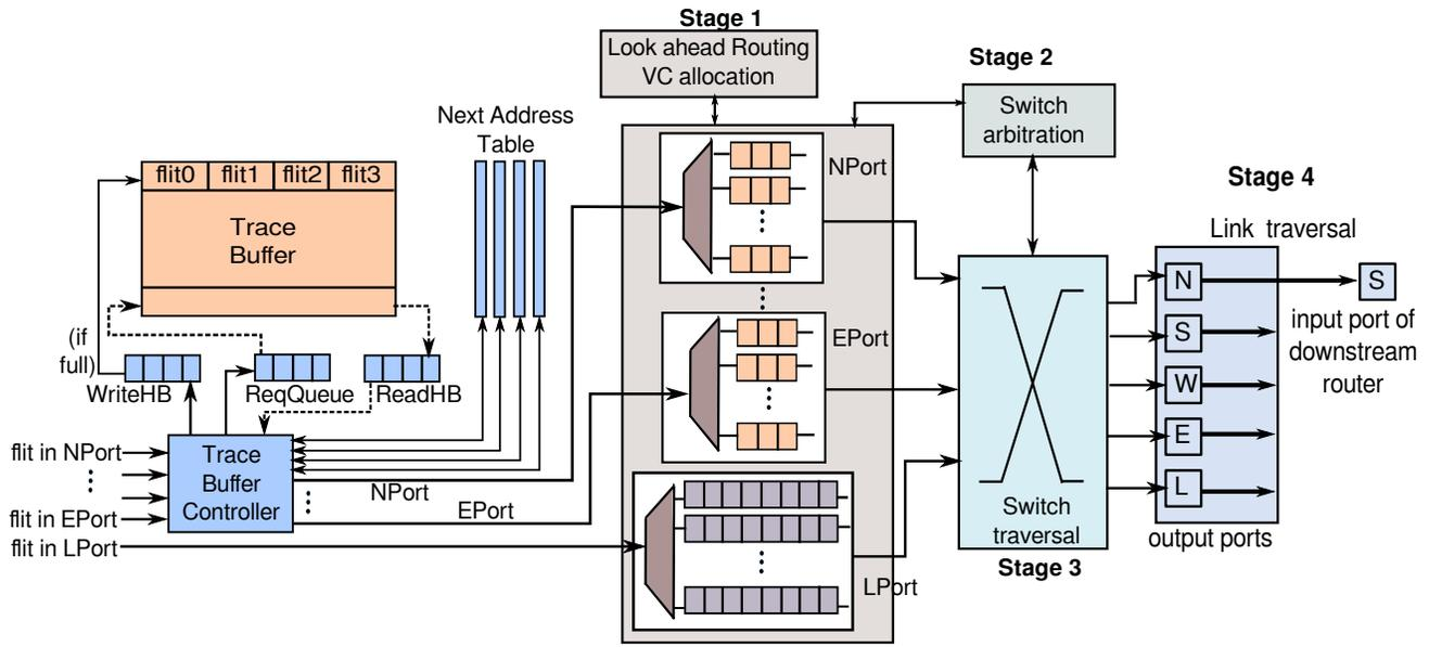
Fig. 3: AugVC Router Architecture
