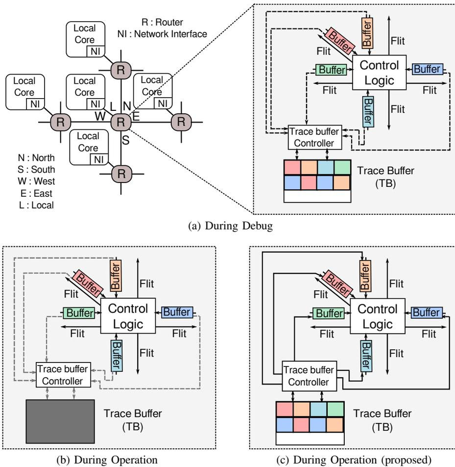
Fig. 1: Trace Buffer reused to augment router buffers.
