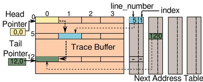
Fig. 4: Linked list of all the flits belonging to the same VC maintained using Next Address Table
