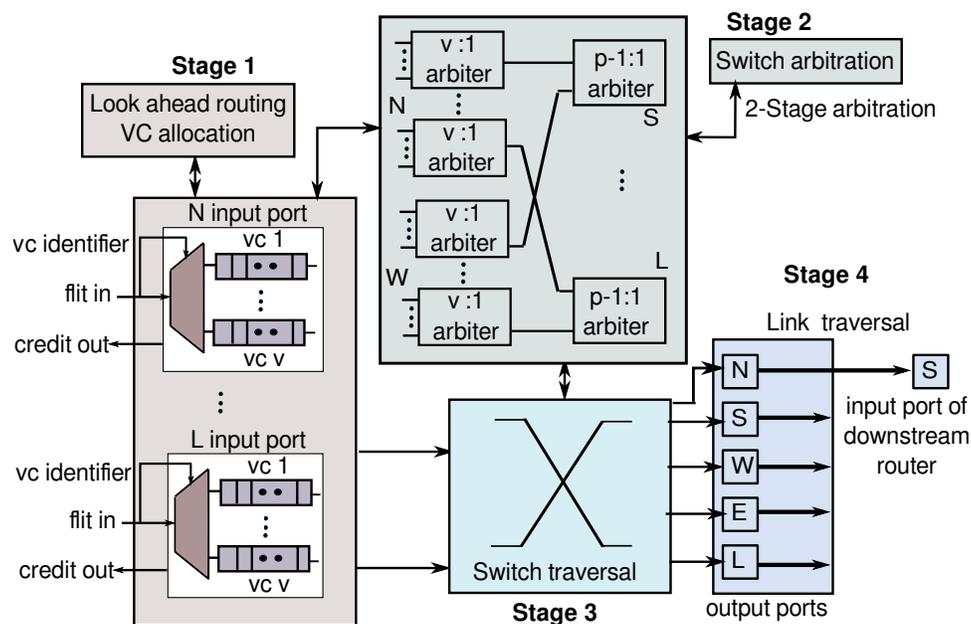
Fig. 2: Conventional Router Architecture.
